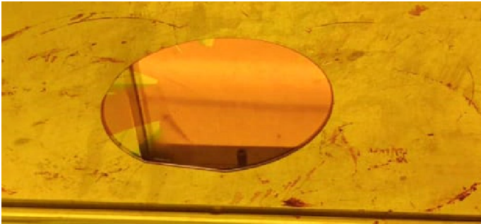
Fig. 9. Wafer spincoated with LOR3A showing non uniform coverage of the wafer.
