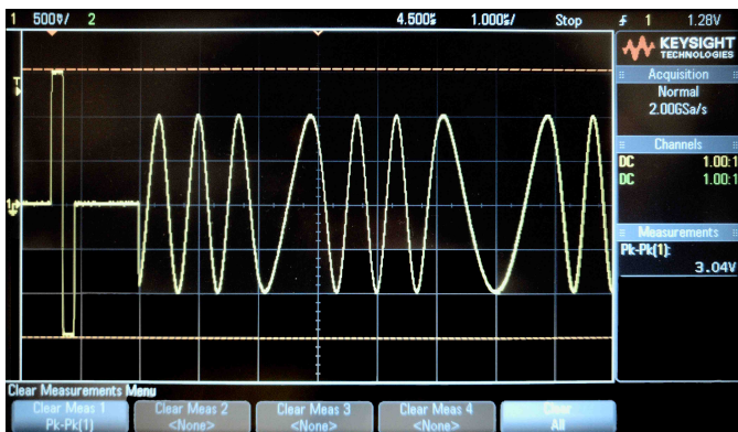
Fig. 10. Oscilloscope acquisition of output from GFSK wave generation.
