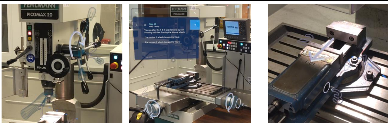
Fig. 1. Different examples of using numbers to indicate operation steps of the PICOMAX. The operation steps shown are Changing machine chug (Left), Referencing the Axis with the manual wheels (Middle) and Changing the size of the Clamp (Right). The numbers are also displayed on the instruction screen, indicating what needs to be done at the place of the number.
