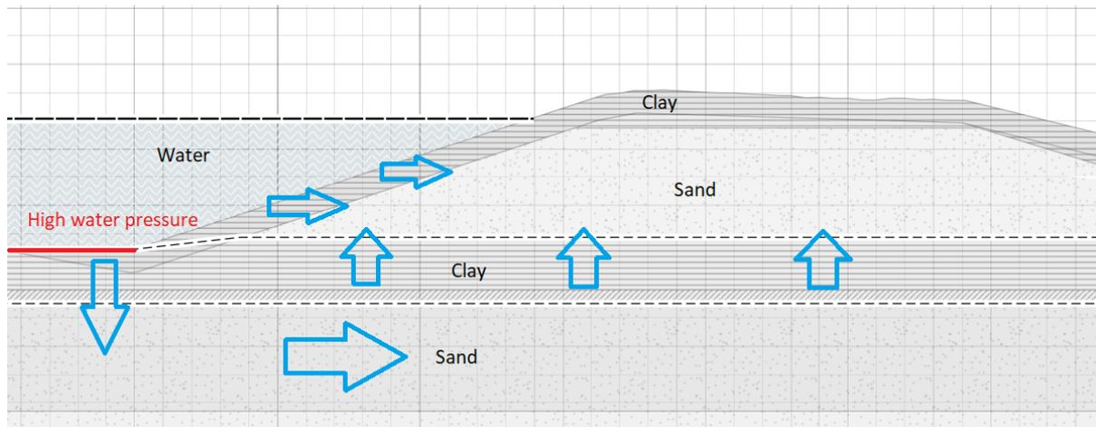
Figure 4, Example groundwater flow in a dike (Deltares, 2023)
