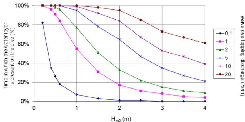
Figure 12, Relation between the percentage of time for which a layer of water is present on the dike and the significant wave height, for several wave overtopping discharges (van Hoven, 2016)
