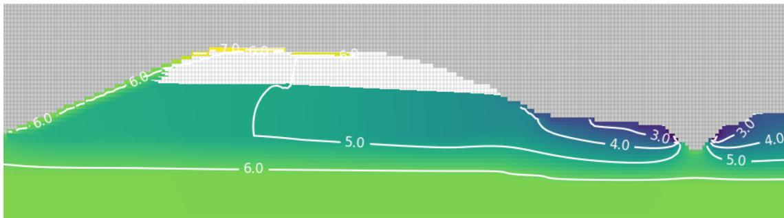
Figure 27, Phreatic line of the dike with thin clay covering on the crest and inner slope
