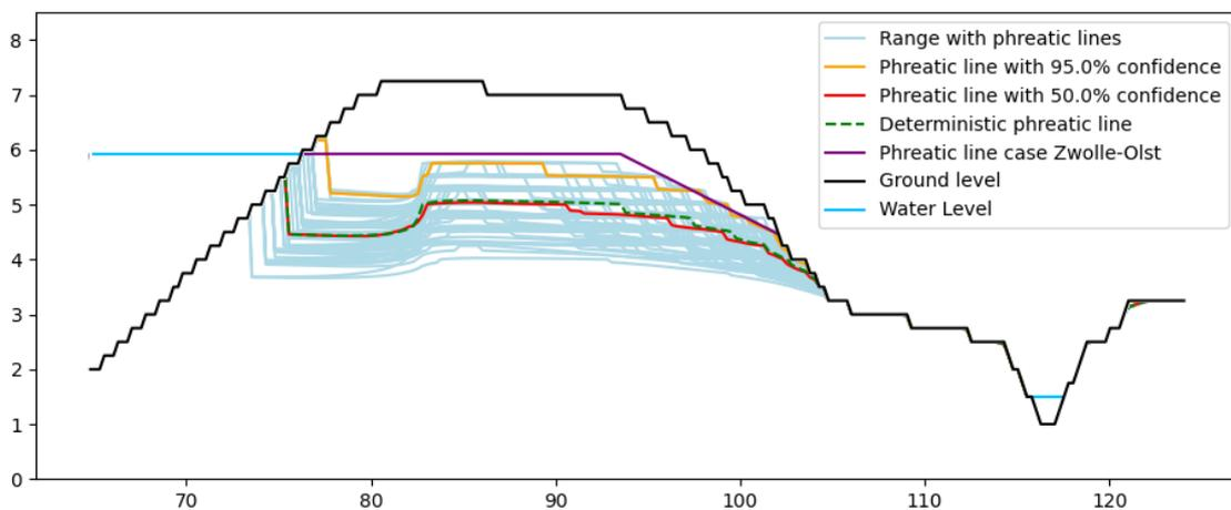
Figure 26, Comparison phreatic lines for  $T=3$  hours
