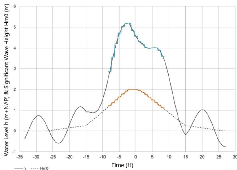
Figure 10, Example of a high water level course, where the solid line is the water level (van Hoven, 2016)
