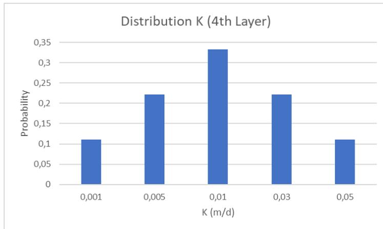
Figure 45, Distribution of the hydraulic conductivity of the fourth layer
