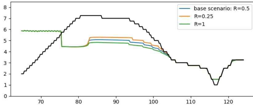
Figure 20, Sensitivity of the phreatic line to a change in the resistance factor
