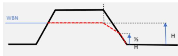
Figure 8 Phreatic line schematization for the case Zwolle-Olst (Klop & van Meekeren, 2021)
