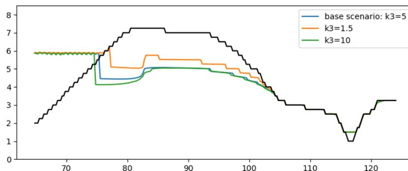
Figure 19, Sensitivity of the phreatic line to a change in hydraulic conductivity of the sandy core
