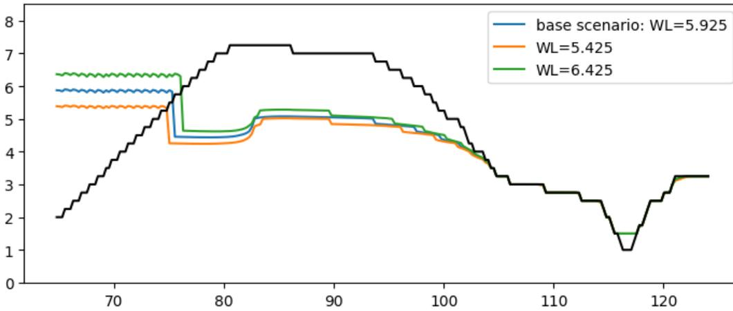
Figure 41, Sensitivity of water levels
