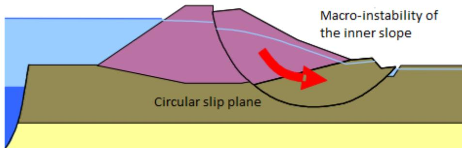
Figure 5, Macro-instability of the inner slope ('t Hart et al.,2016)
