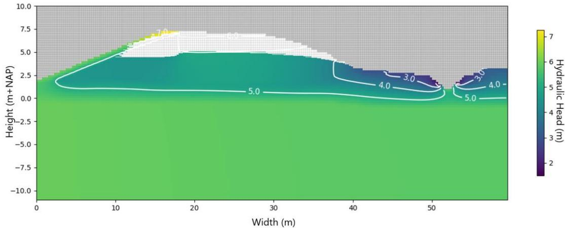
Figure 17, Cross-section model output with the effects of wave overtopping (T=3)
