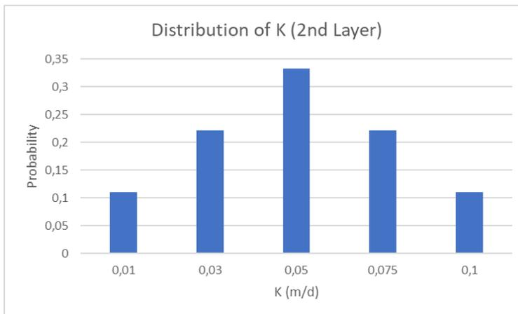
Figure 43, Distribution of the hydraulic conductivity of the second layer
