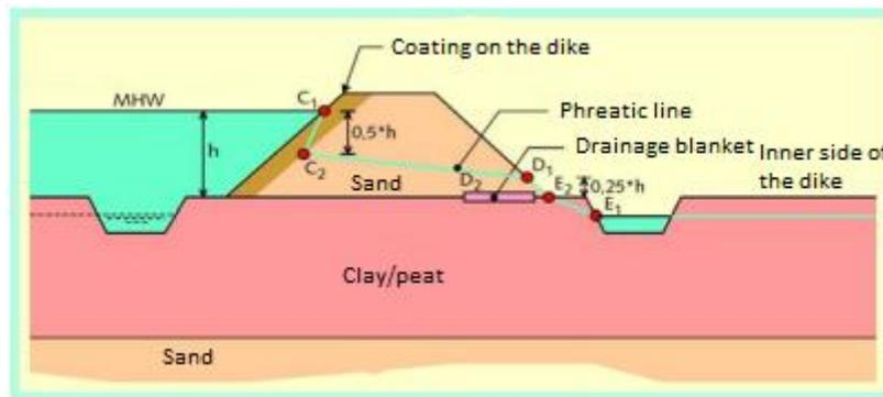
Figure 7, Schematization of the phreatic line for a sand dike with a clay or peat soil layer below the dike (low overtopping discharge) (TAW, 2004)
