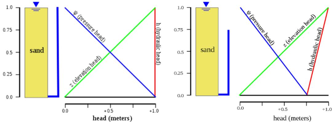
Figure 3, Example of the difference between hydrostatic and not hydrostatic (Linquip TechNews, 2020)
