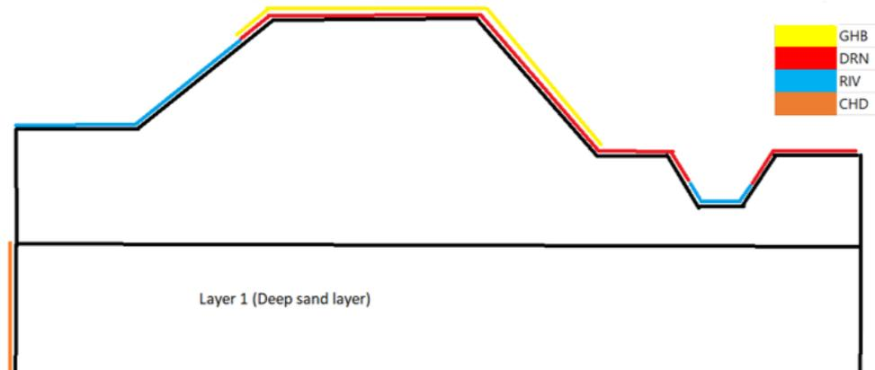
Figure 30, Location of some packages within the cross-section
