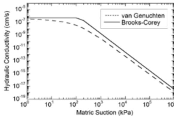
Figure 9, Comparison van Genuchten and Brooks & Corey (Schanz, 2007)
