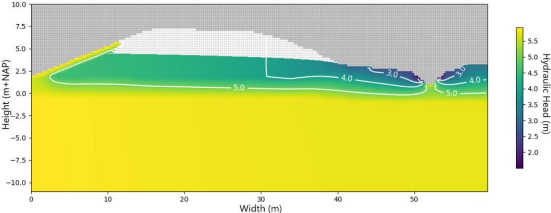
Figure 16, Cross-section model output without wave overtopping (T=0)
