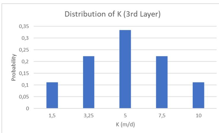
Figure 44, Distribution of the hydraulic conductivity of the third layer
