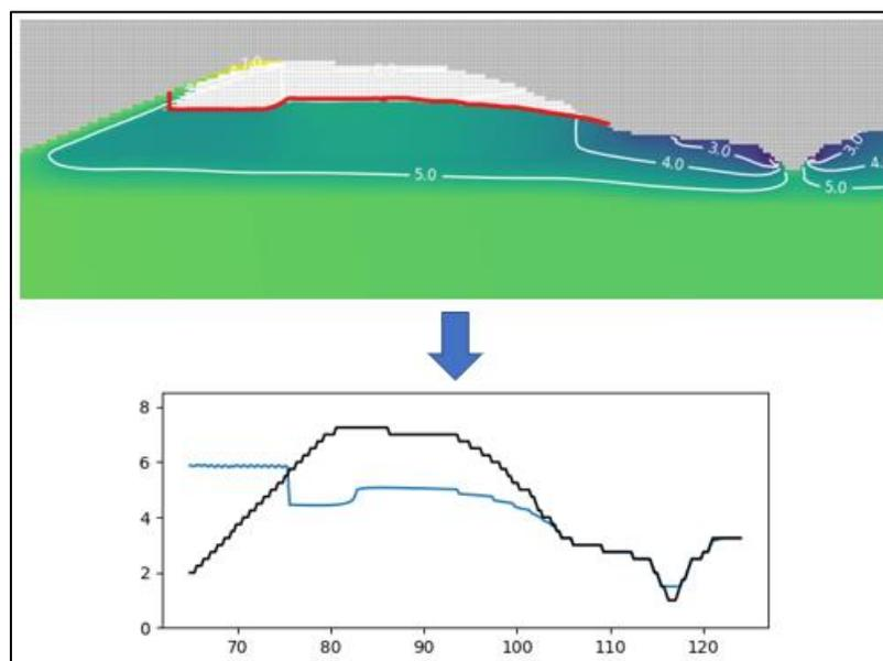
Figure 18, Process of storing the phreatic line as a CSV and using the CSV to plot the phreatic line
