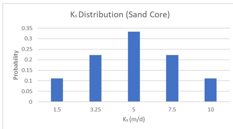
Figure 21, Distribution of possible hydraulic conductivities of the dike's sand core
