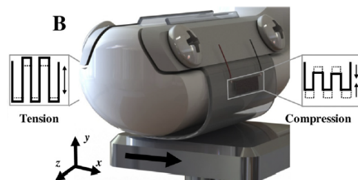
(b) Sensor design from Yin et al. [35] where tension and compression from shearing are measured using piezoresistive gauges.
