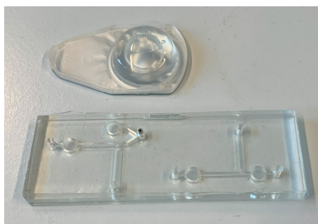
Figure 7: The set-up of the experiment using an eye lens to mimic the blister pouch with a blunt needle glued in the inlet.
