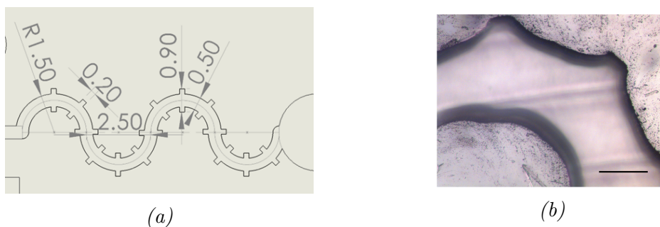
Figure C.11: The serpentine mixing structure with side wells: a technical drawing with top view (a) and under the microscope with magnification 40x (b) scalebar = 500 \mu\text{m} .
