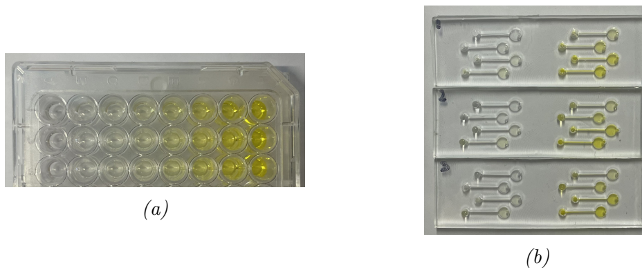
Figure 33: A picture of the calibration curve measurements in triplo on a wells plate (a) row A,B,C with increasing concentration colomn 1-8, and in microfluidic devices (b) with increasing concentration from top left to bottom right.
