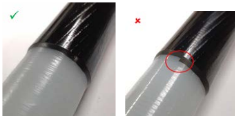
(a) Fluent transition. (b) With sharp corner.
