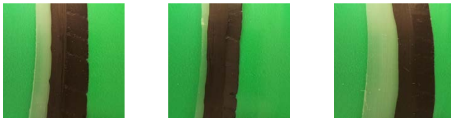
(a) Proper blade depth Q \approx 0 (b) Too shallow Q > 0 (c) Too deep Q > 0
