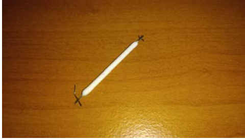
Figure 10: Picture of a LED bar taken from a commercial LED filament bulb.
