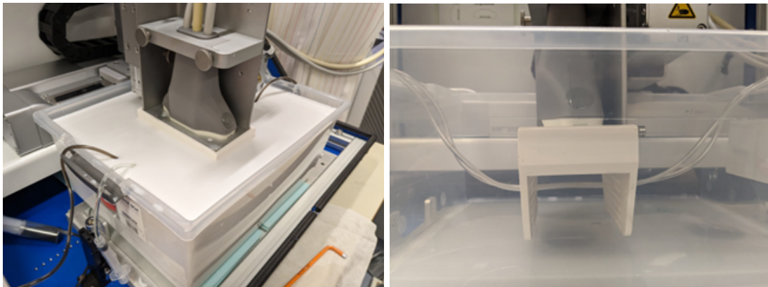
Figure 2.6: Pictures depicting the experiment configuration with a filled water bin (left) and an empty bin (right) to visualise the tubes with regard to the holder and transducer positions.
