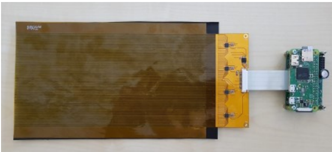
Fig. 4: Pressure sensor, acquisition board, and Raspberry Pi Zero W
