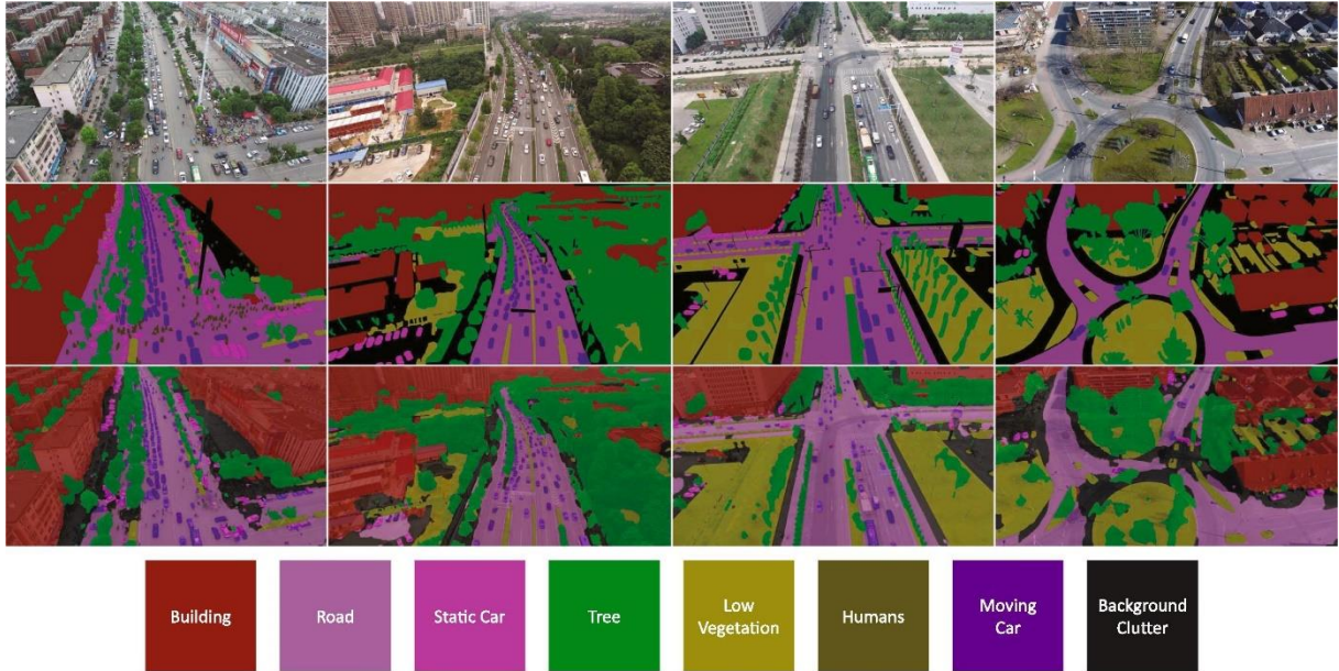
Figure 17: Illustration of different classes with their assigned colour from the UAVid dataset. Original images, ground-truth labels, and predicted labels in first, second, and third row, respectively. ( uavid.nl )
