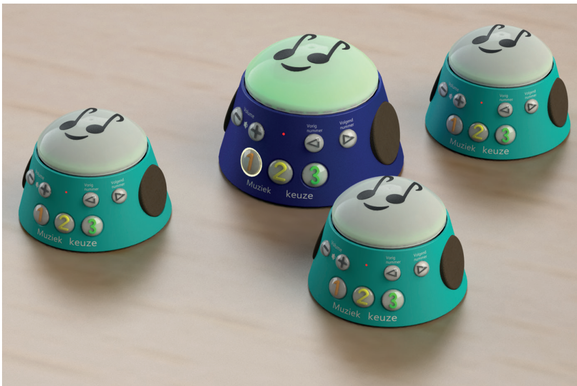
Fig. 45. A network consisting of the hub and three stations, the hub is turned on and playing music choice 1.
