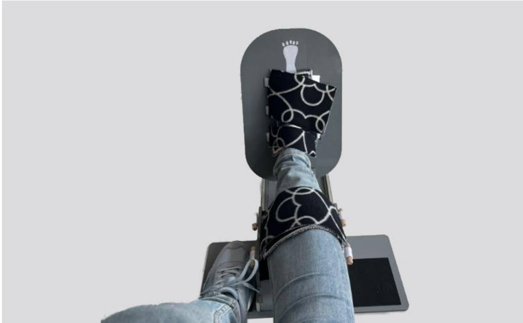
Figure 29. Foot and lower leg fixated in the 3D stress foot plate device. There are three attachment straps; one at the lower leg, and two at the foot.
