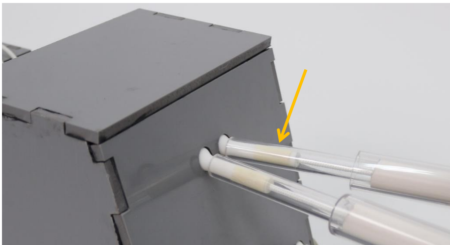
Figure 22. Close up of the ball-and-socket joint. Since the PMMA inner tube was loosely wrapped around the joint, some tape was placed around the stick of the joint, which can be seen with the yellow arrow.
