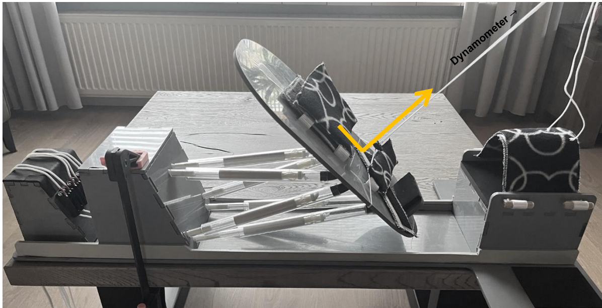
Figure 28. Set-up for measuring tensile force of the foot plate, the device is fixated in a slightly plantarflexion position. It is indicated, that an attempt was made to get the force perpendicular to the foot plate.
