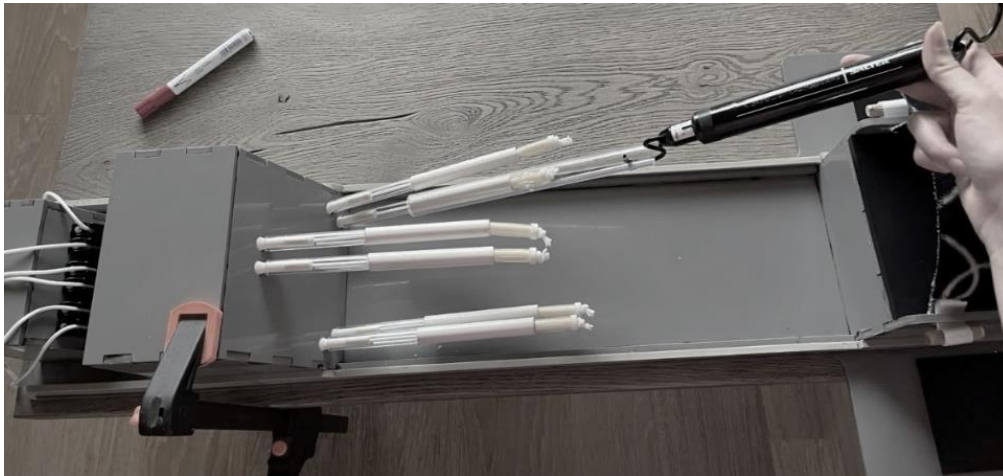
Figure 27. Test set-up for measuring the tensile force.
