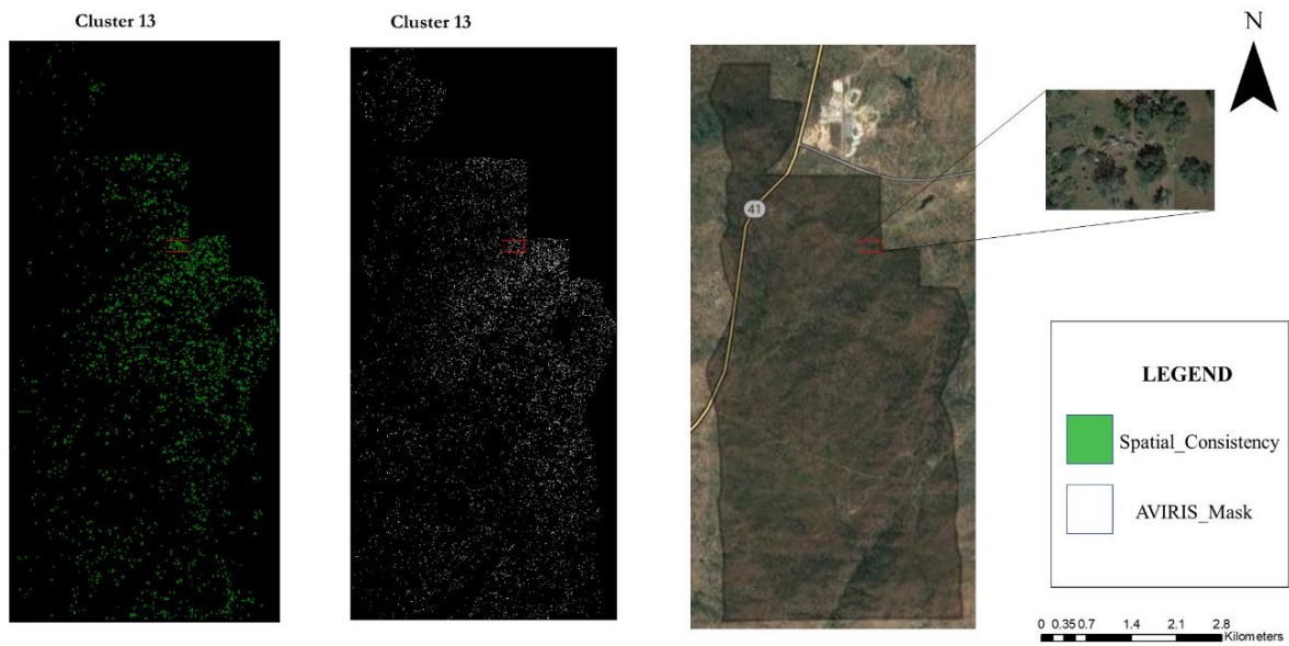
Figure 40 Spatially Consistent Clusters in Spatially Upscaled 16m Image And AVIRIS-NG together with a Corresponding Region In High Resolution.
