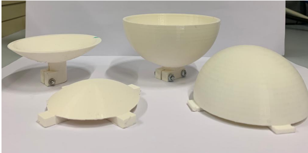
(a) Side view of inner and outer molds of sample molds (left) and phantom molds (right).
