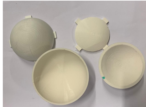
(b) View from above of inner and outer molds of sample molds (right) and phantom molds (left).
