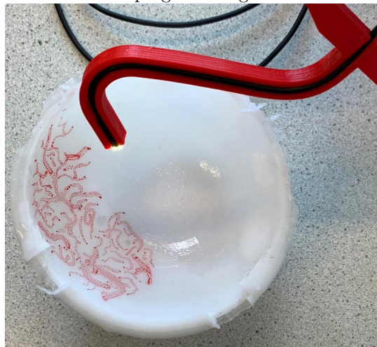
Figure 9: Miniature camera used to image blood vessels on phantom BP2.
