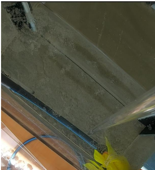
Figure 6.1: Top view of soil deformation in standard heave experiment
