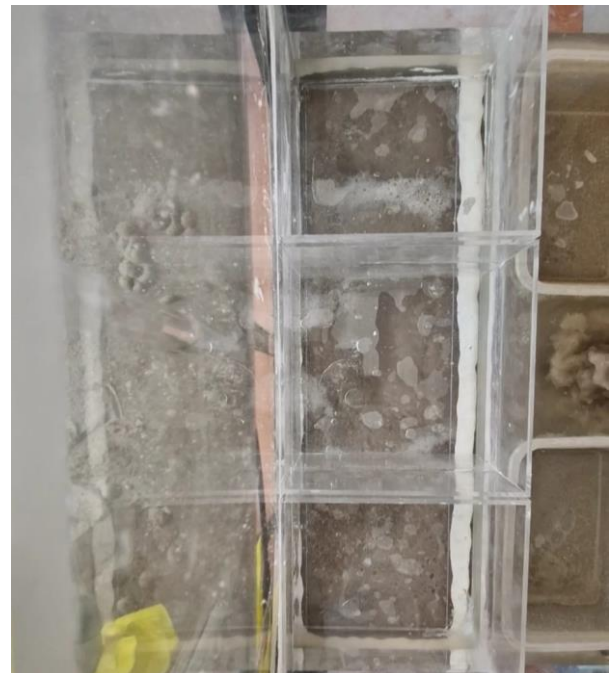
Figure 6.2: Top view of the moment of the soil aggregate outburst in heave experiment 6 (2,2 kg)
