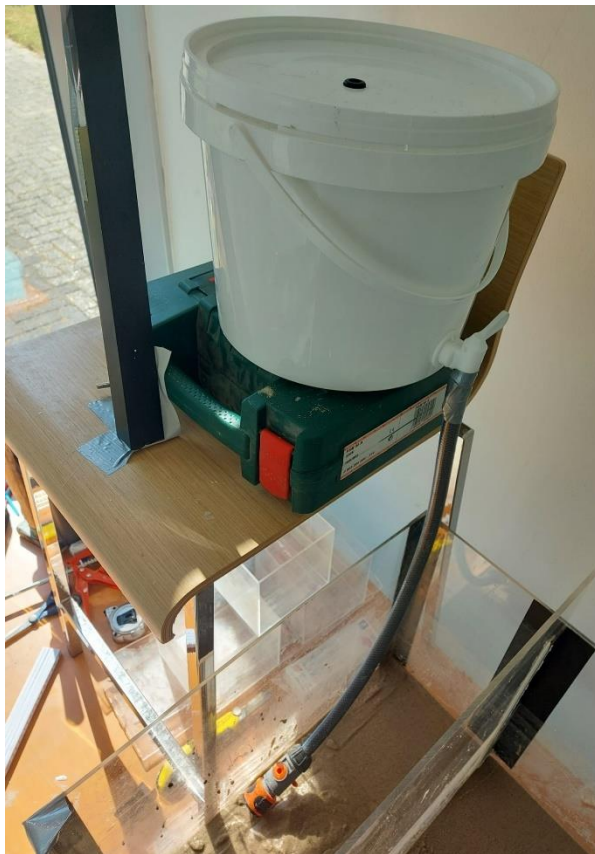
Figure 5.6: Water inlet with bucket and hose
