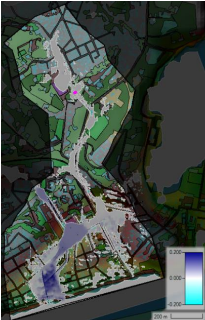
Figure 48 – Inundation difference map of the southern drainage system for scenario 18
