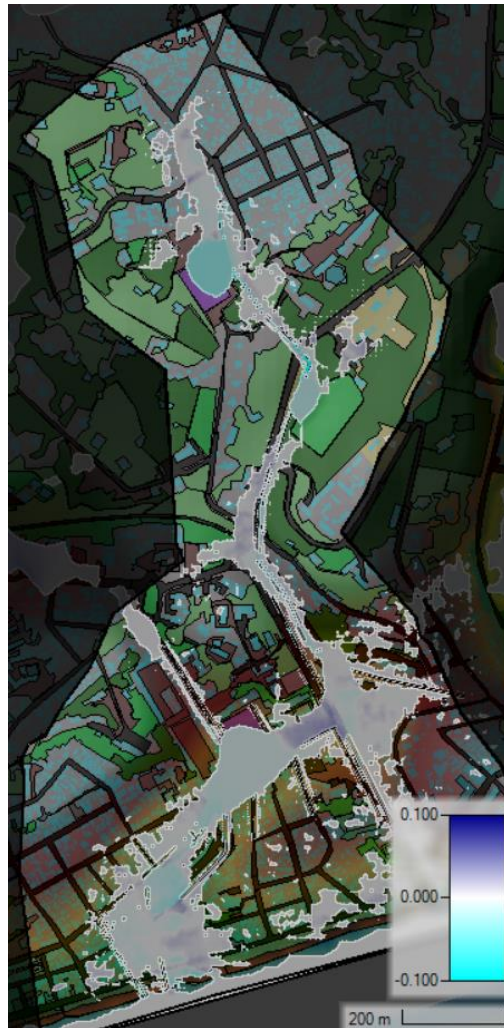
Figure 97 - Comparison inundation map of the whole catchment for permeable pavement implementation
