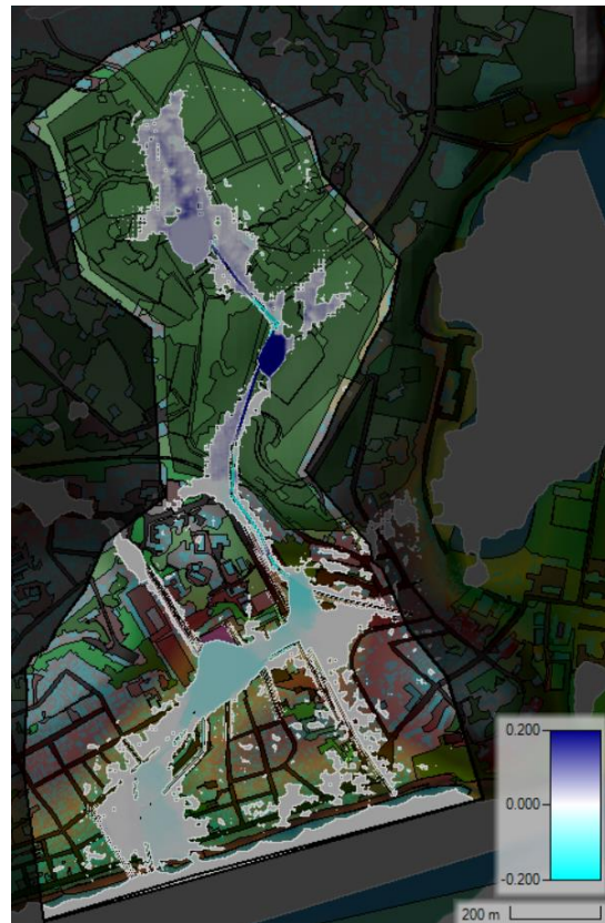
Figure 79 - Inundation map in comparison to the original situation, when the northern part consists of forest
