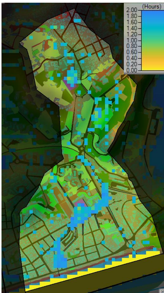
Figure 16 - Duration before water depths exceed 10 cm per location
