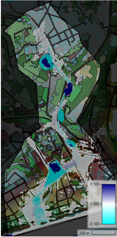
Figure 93 - Comparison inundation map with bioswale implementation for the whole catchment
