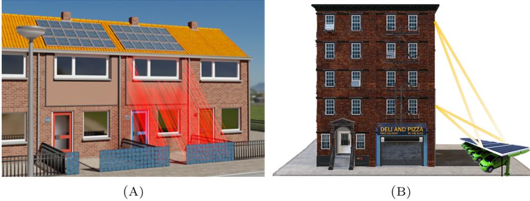
FIGURE 1.5: Applications of an FSLSC showing A) a two-story residential façade with a bifacial fence and B) a five-story façade with a bifacial car shed. Figures from [8].
