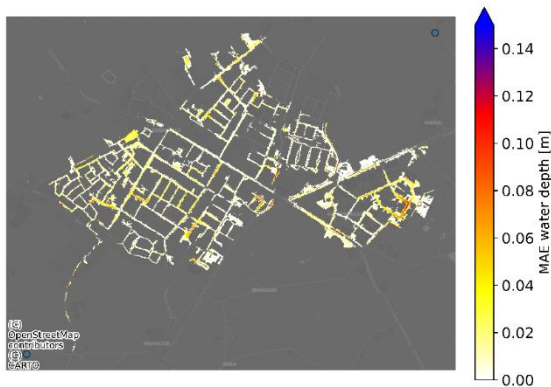
Figure 18 - Mean Absolute Error (MAE) over the 8 validation runs. The predicted water depth according to the ML model is compared to the hydrological inundation model output.
