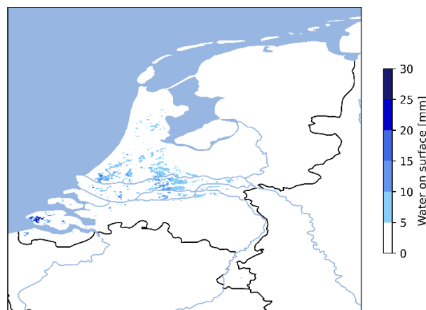
Figure 46 - Output of the W2O model for 09-09-2022 at 06:00. Water on surface level [mm] for the 90 th percentile of all ensemble members. The maximum over time is taken for each grid cell.
