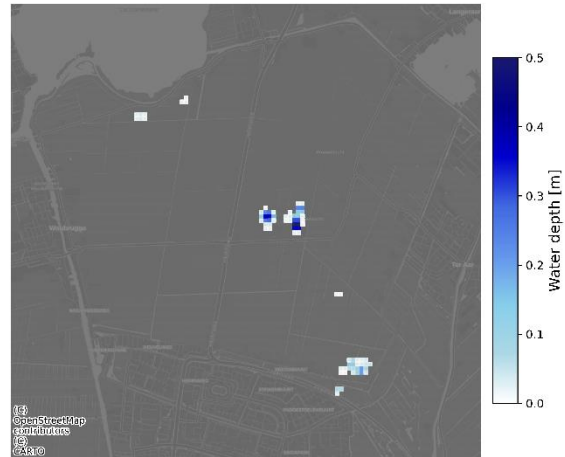
Figure 38 - Output of the surrogate model: maximum water depth over time on the 2D grid for the 90 th percentile of ensemble members.
