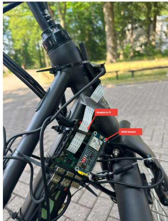
Fig. 5. Raspberry Pi and GNSS module setup
