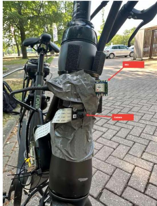
Fig. 4. Camera and IMU setup
