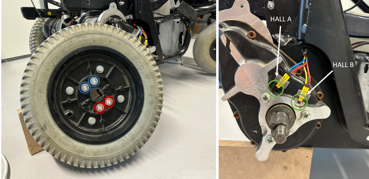
Figure 15: Placement of the magnets and hall sensors on the wheelchair.
