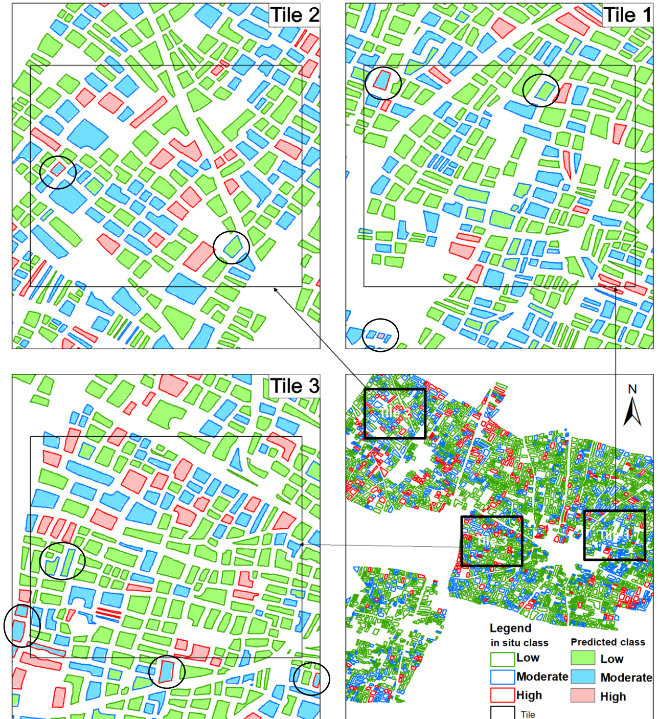
Figure 20. Majority pixel classification of combined (S1 and S2) damage class prediction output.
