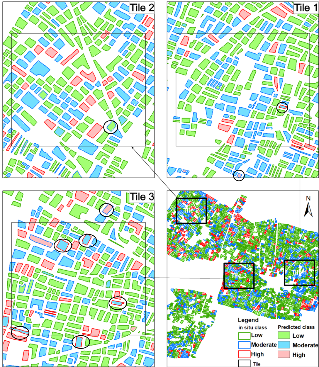
Figure 23. Combined (S1 and S2) damage class prediction output of OBC (experiment 6).
