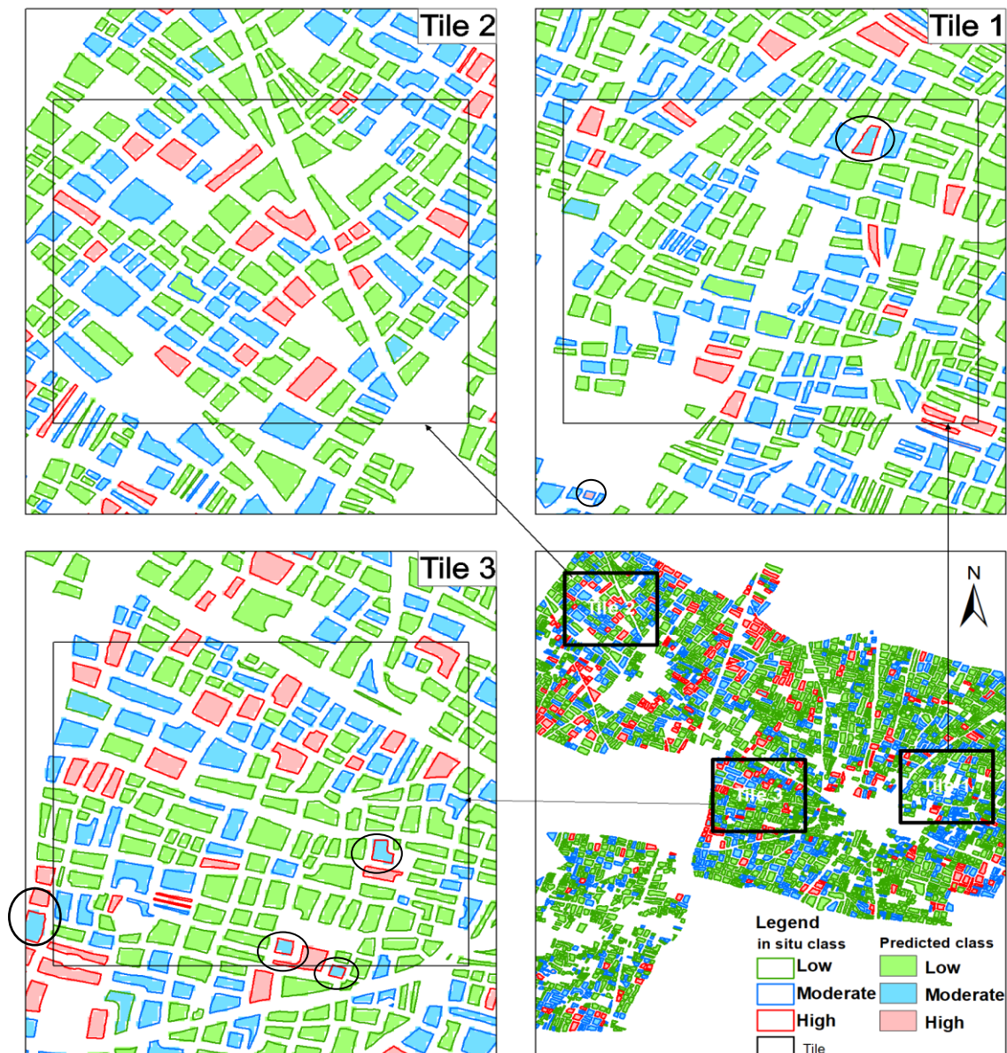
Figure 21. Sentinel-1 damage class prediction output of OBC (experiment 4).
