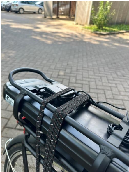
Fig. 2. The GNSS-RTK sensor on the back of the bicycle
