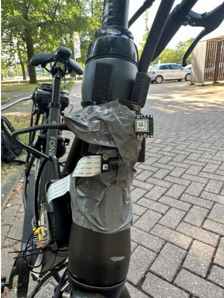
Fig. 1. The camera with the Raspberry Pi on the front of the bicycle
