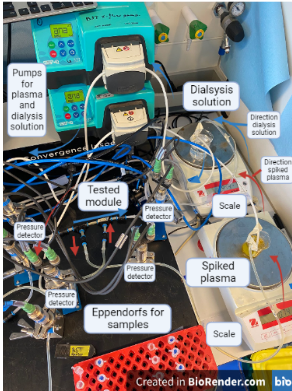
Figure 21: Performing a toxin removal experiment using the Convergence set-up.
