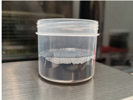
Figure 3.5: 15 g of Ecoflex part B (clear) added to 3.5 g of filtered powdered Vulcan XC72 (black)
