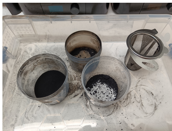
Figure 3.4: Separation of powdered filler using a tea sift
