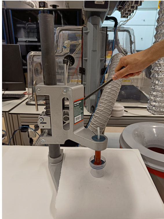
Figure 3.13: Developed tool for loading a syringe with mixed materials
