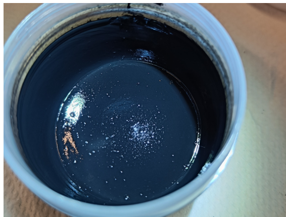
Figure 3.6: Dispersion of Vulcan XC72 and Ecoflex 00-30 (mass fraction of 10.5 %)
