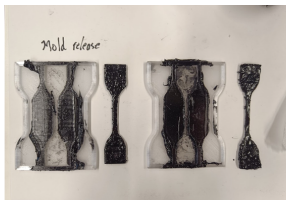
Figure 3.17: A silicone part cast in a mould with and a mould without Mann easy release 200
