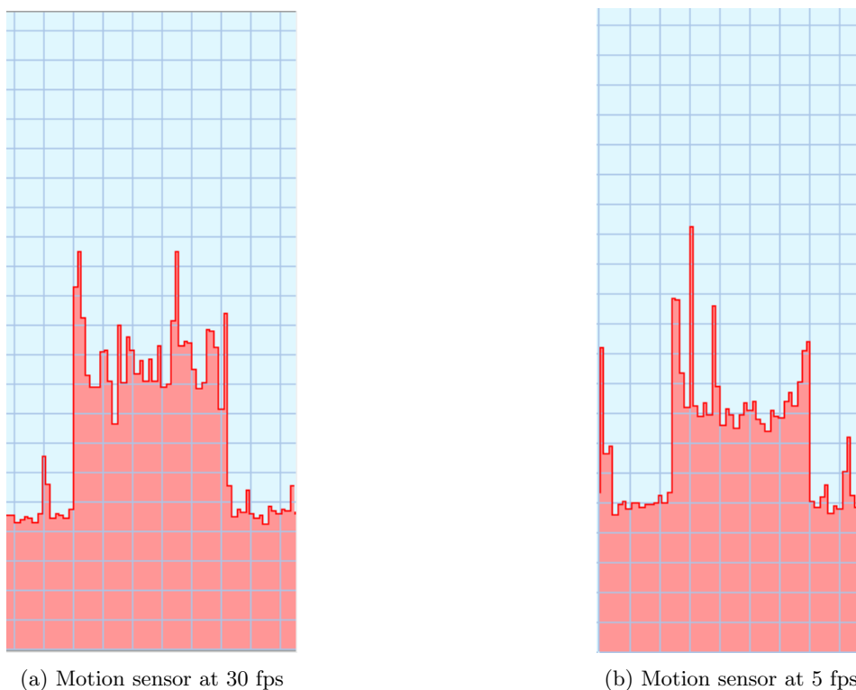
Figure 6.3: Motion sensor power consumption comparison
