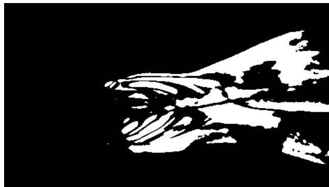
Figure 5.1: Perspective of motion detection model. White pixels show the difference in brightness between two consecutive frames that exceeded the threshold filter.
