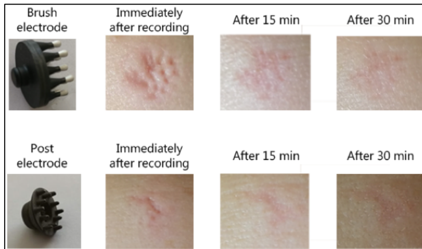
Figure 8: "Skin irritation for short term use of dry electrodes. In the top: Post electrode with pins of 2 mm length; At the bottom: Brush electrode with pins of 5 mm length" [28, p.3]
