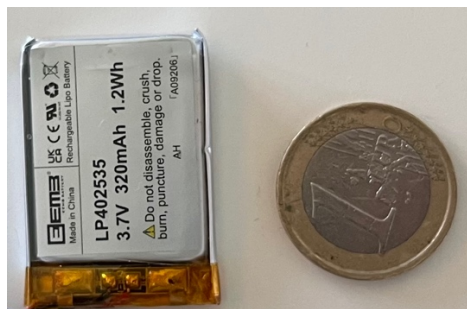
Figure 20: Lithium-Polymer Battery size comparison 1€ Coin
