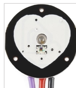
Figure 19: PPG sensor, no protrusion [36, p.1]
