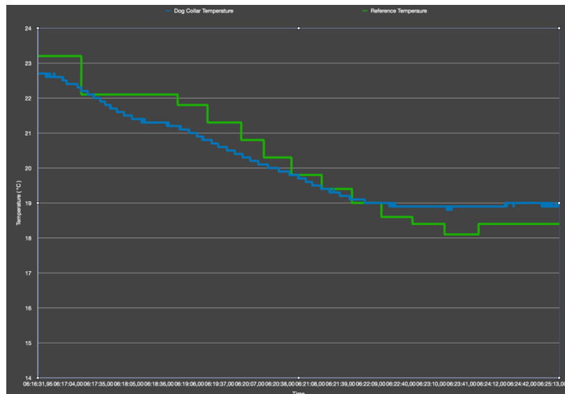
Figure 38: Temperature measurement comparison of Prototype and other Thermometer
