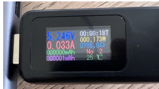
Figure 45: Power Consumption, Bluetooth OFF
