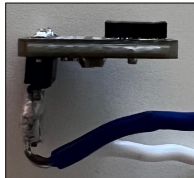
Figure 17: Protrusion of the Sensor (black component)
