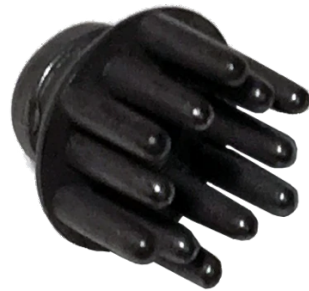
Figure 7: Dry Electrode with extended prongs, end of prongs touches the skin [27]
