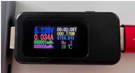
Figure 44: Power consumption, Bluetooth ON
