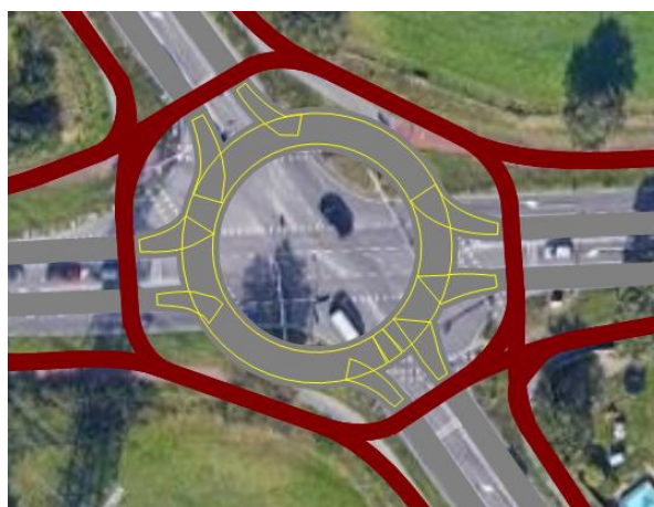
Figure 9: Reduced speed zones on roundabout
