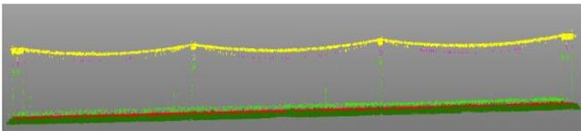
Figure 10 Contact cable detection using DBSCAN highlighted as purple points
