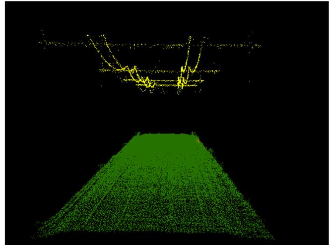
Figure 7 Cross sectional view of the applied coarse classification on the dataset
