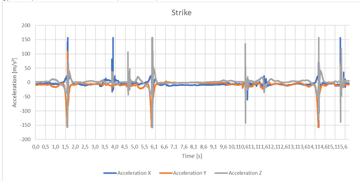
Fig 11: Acceleration in X, Y and Z direction during field hockey strike.
