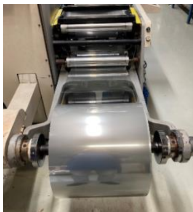
Figure 8: Plastic production roll attached to the unwind guide
