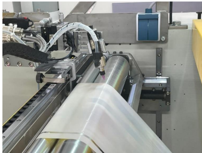
Figure 15. Tetrahydrofuran being applied to the substrate
