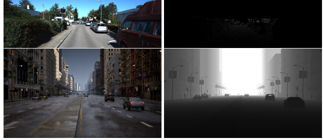
Figure 8. RGB-depth pair for both KITTI (top, sparse depth) and the virtual data set (bottom, dense depth).
