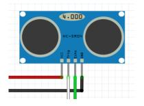
a signal. See figure 40 for the wires connected to the ultrasonic sensor.
