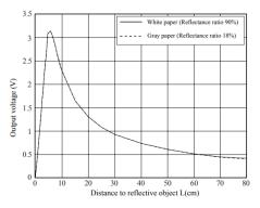
Figure 35: Distance measuring characteristics GPY0A21YK0F infrared sensor
