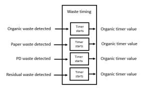
Figure 26: Level 2 waste timer black box model
