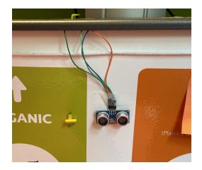
Figure 45: The ultrasonic sensor placed on the outside of the waste island
