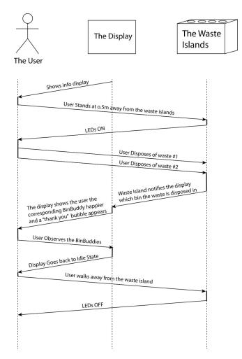
Figure 28: Time sequence diagram 1
