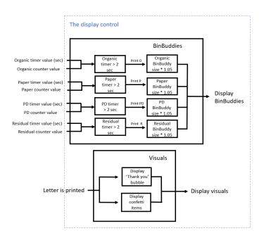
Figure 27: Level 2 display control black box model
