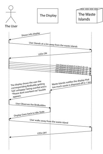
Figure 31: Time sequence diagram 4
