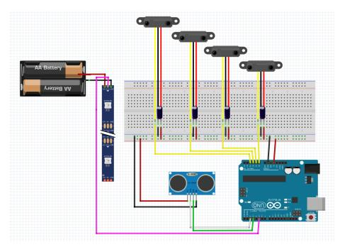
Figure 37: The integrated hardware
