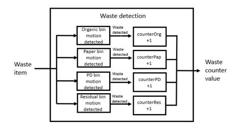
Figure 25: Level 2 waste detection black box model
