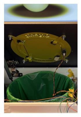
Figure 44: The placing of the infrared sensors
