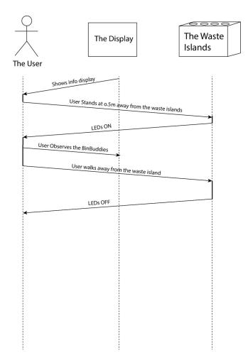
Figure 29: Time sequence diagram 2
