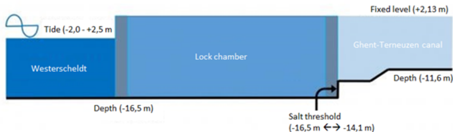
Figure 2.5: Schematic representation of New Lock Terneuzen and salt threshold (source: nieuwesluis-terneuzen.eu)
