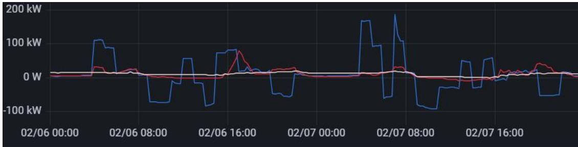
Fig. 5.7: neighbourhood meter using different control algorithms: Profile steering (yellow), no control (red) and price steering (blue)
