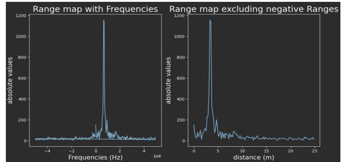
Fig. 3. Range map of 1 chirp with frequencies and distances
