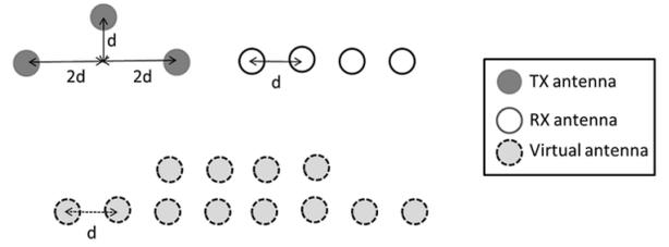
Fig. 1. The 2D antenna MIMO array
