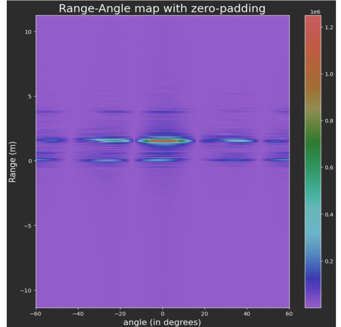
Fig. 5. The Range-Angle map at candidate Velocity
