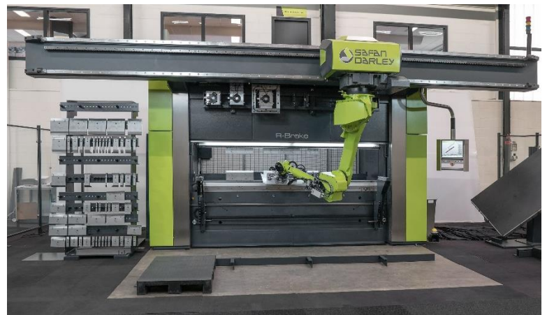
Safan-Darley R-Brake automated bending cell using the WILA ATC system.
