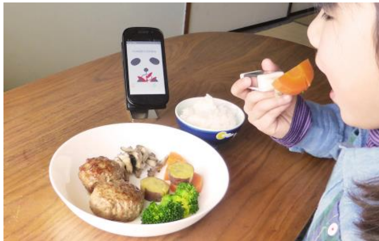
Figure 4: Sensor embedded fork
