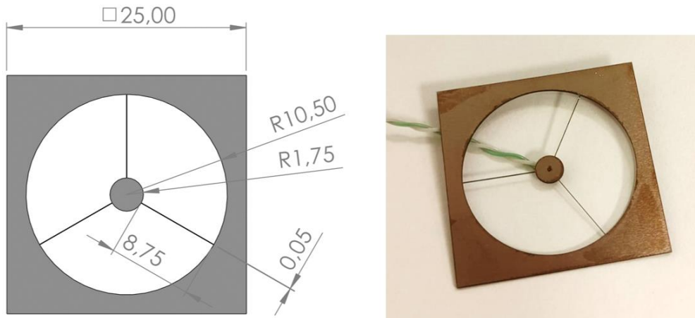
Figure 16: Sample made out of 0.3 mm AISI 420 hardened steel. Left: dimensions of the sample in mm, right: physical sample with attached thermocouple with green-white wire.
