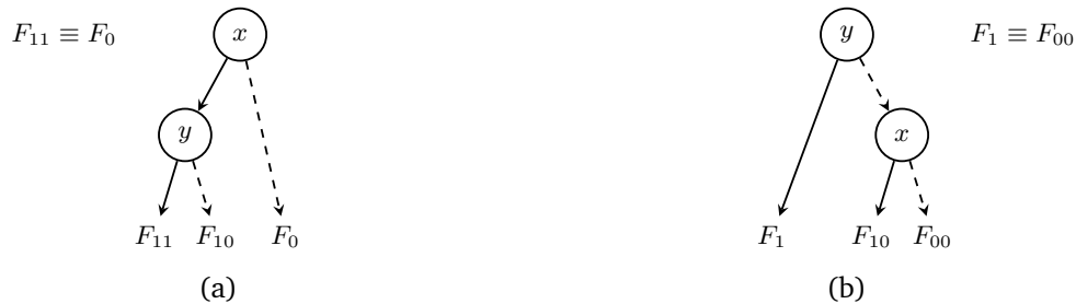
Figure 2.8: Variable swap between x_1 and x_2 resulting in the same number of nodes
