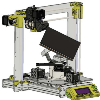
(a) Parallel manipulator for Prusa MK3[49]
