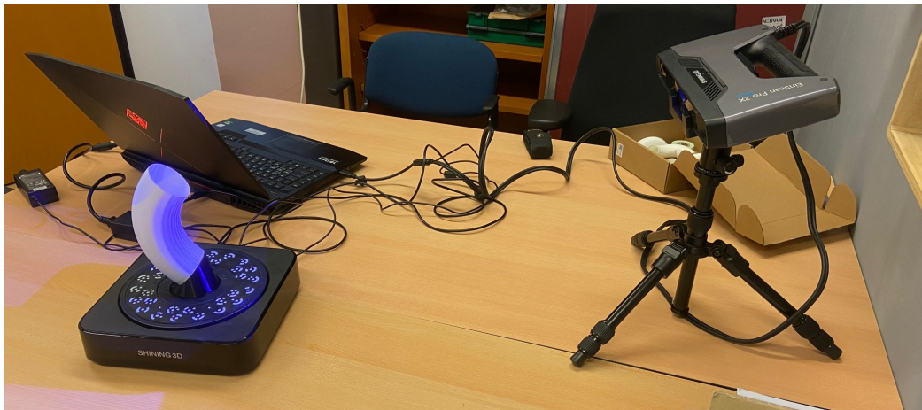
Figure 5.4: Setup for dense point 3D scanning with EinScan Pro 2x industrial kit
