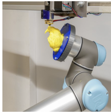
(b) Build-plate on end effector[47]
