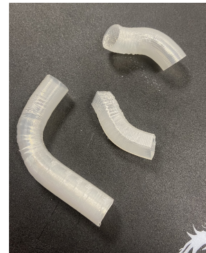
(c) Swept profiles printed with VP1
