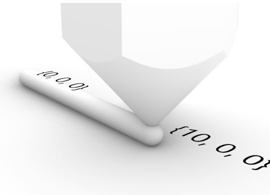
Figure 4.3: Deposition of a single track of material by giving a G-code command.
