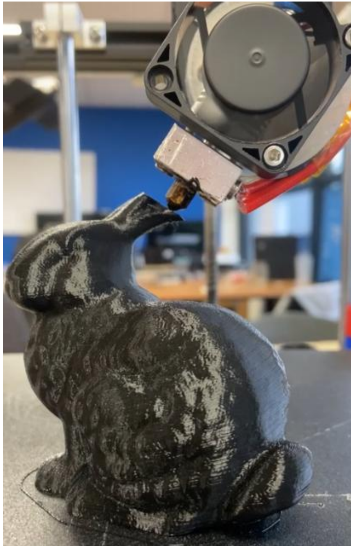
Figure A.7: Stanford bunny[100] being printed using G-code bending
