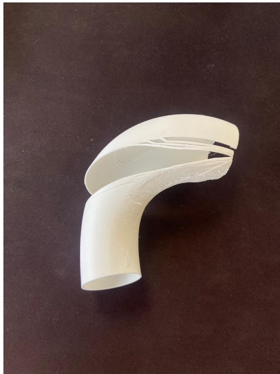
Figure A.4: Planar sample part broken during support-removal
