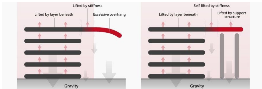
Figure 1.12: Principle of using support structures as scaffolding for overhanging geometry[18]
