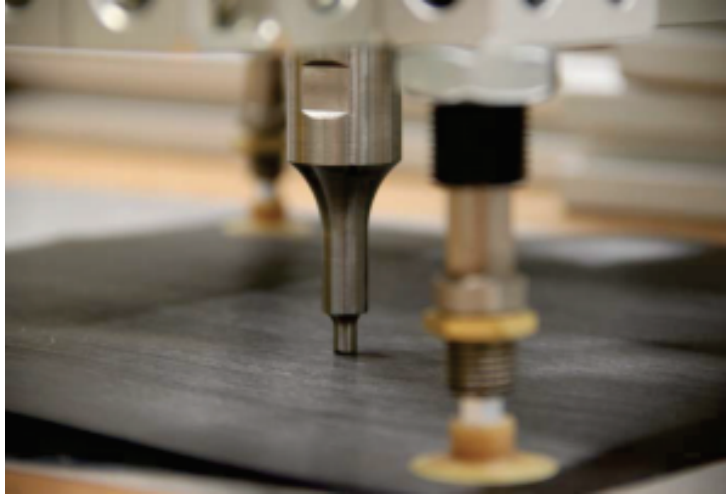
Figure 4.4.4: Spot welding after placement by vacuum grippers [14]
