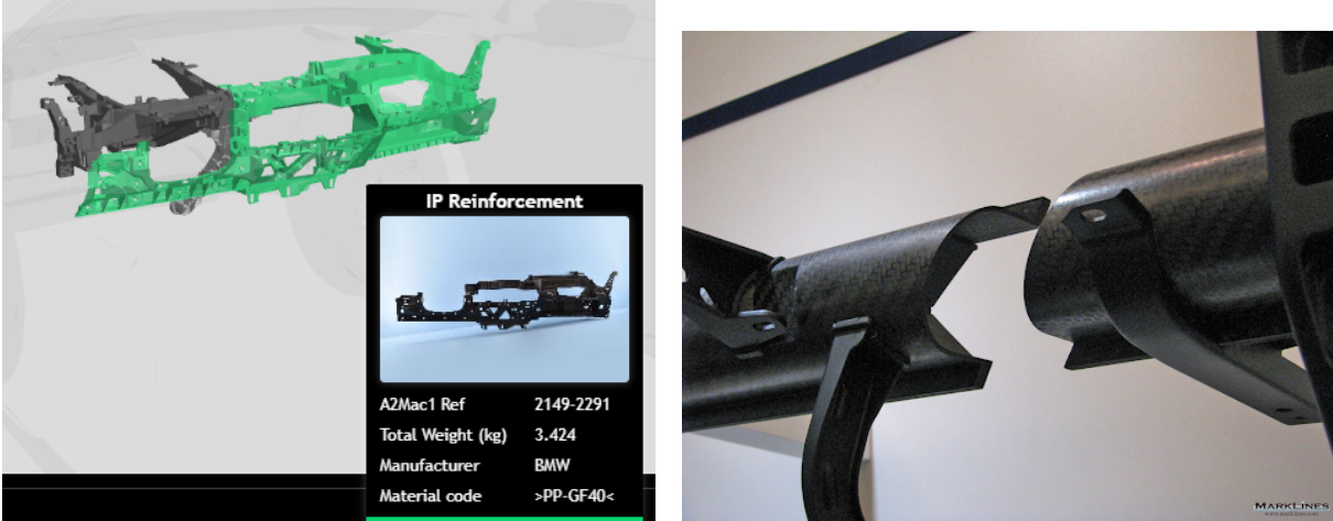
(a) Half composite CCB concept in the BMW ix drive 50 sport 2022 [3] (b) Concept of a press formed composite CCB by Faurecia [41]
