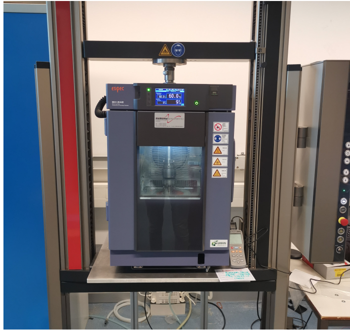
(b) The climate chamber regulating the temperature and relative humidity around the sample and the H-like frame of the tensile machine around it
