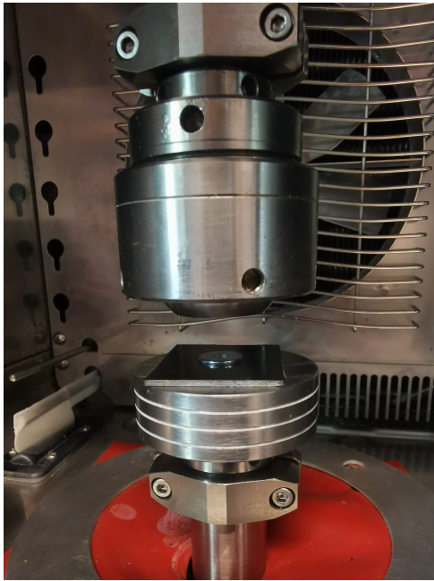
(a) The relaxation setup with the specimen and washer between the heads of the tensile testing machine
