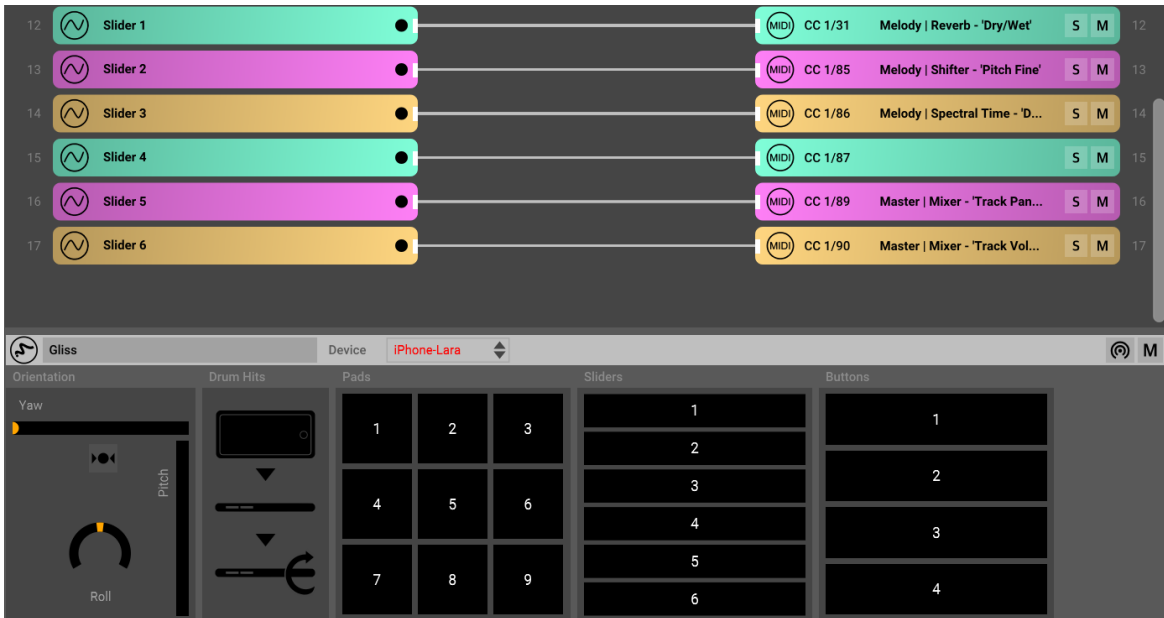
Figure B.1: A snapshot from the Glover software (Version 1.1.2; MI.MU Gloves Limited, 2010). There, you can see an example set of inputs' (i.e. different sliders from an app interface) representation ( Left ), as well as their connection to various sound change/effect outputs to a software that allows for music creation ( Right ). The below part shows real-time data from the app that movements inputs come from.
