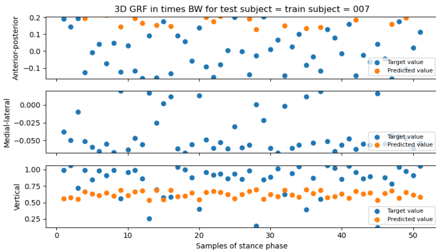
Figure 23 3D GRF predictions of the pyrenn-based model, after rescaling y-axes to the range of target values.
