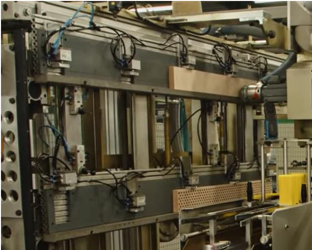
Figure 2-1: Drilling holes and punching brush material in the product
