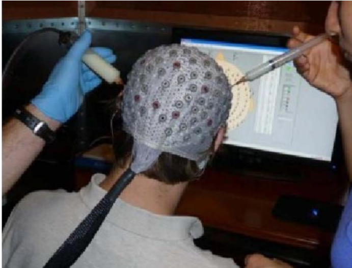
Figure 7: Exemplary depiction of the wet electrode system adopted from Nathan et al. (2013).
