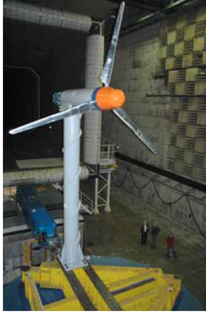
Figure 4.1: Set-up of the MEXICO experiment [23]
