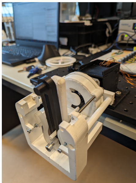
Figure 4.11: Prototype realization of multi-axis motor integrated VIA
