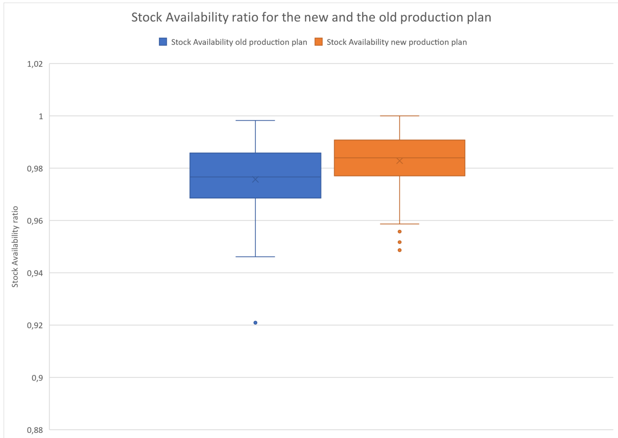
Figure 15: The boxplots that show the Stock Availability ratio for the old production plan and the new production plan using the VMQ-method. The boxplots are made based on the 232 data points, where each data point represents the average Stock Availability ratio of all SKUs over 2023 of a different replication.
