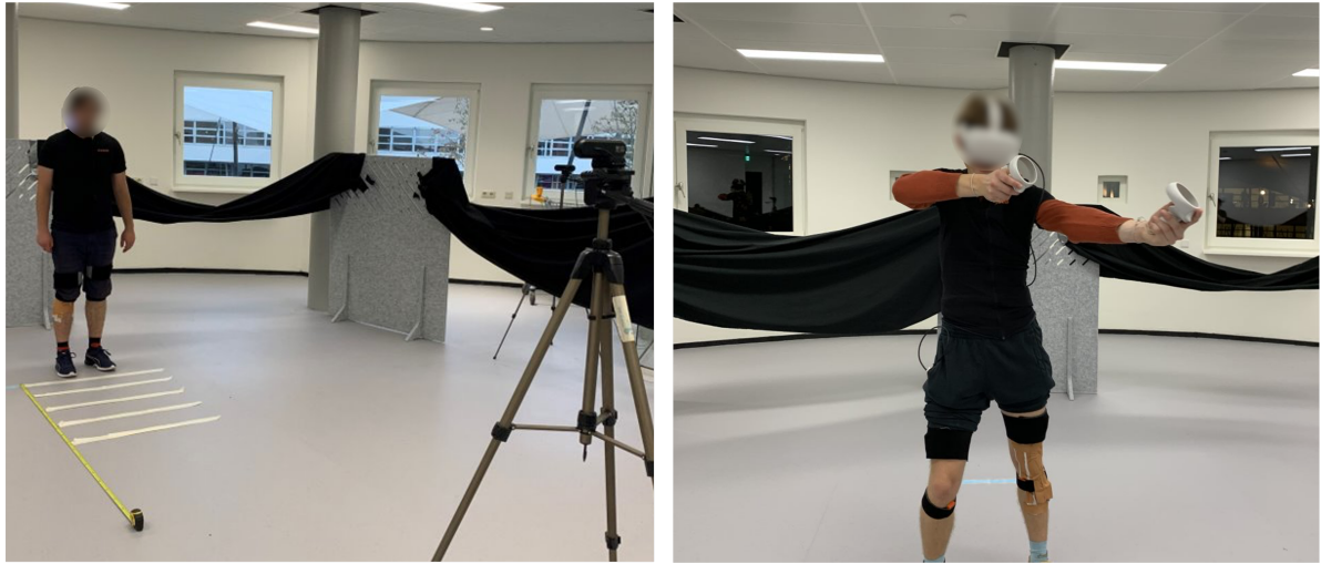
(a) Setup of the additional VR influence measurement in the real-world condition for a participant, including a webcam setup to the front and the side of the participant; the participant should jump at the distances of 20, 40, 60 and 80% of the maximum that connected to a portable charger and holding the Oculus controllers. The MVN sensors are placed on the participant standing ready to jump, with his non-dominant leg perturbed with sports tape. (b) Participant getting ready to play the VR-ACL system in the real-world condition for a participant, including a webcam setup to the front and the side of the participant; the participant should jump at the distances of 20, 40, 60 and 80% of the maximum that connected to a portable charger and holding the Oculus controllers. The MVN sensors are placed on the participant standing ready to jump, with his non-dominant leg perturbed with sports tape. The MVN sensors are placed within the participant's shoes and the sensor attached posteriorly to the pelvis). The participant's non-dominant leg (left) is perturbed with Leukotape P sports tape.
