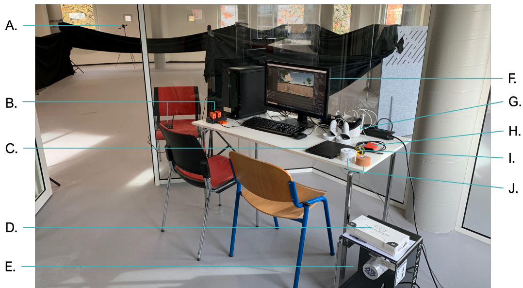
(b) Setup of materials needed for the evaluation, including the video camera (A.), the MVN sensors charging and the MVN Awinda (B.), an iPad for note taking and audio recordings (C.), disposable HMD coverings (D.), VR cleaning box (E.); computer streaming Unity scene and SteamVR (F), Oculus Quest 2 HMD and two controllers (G.), external charger for HMD (H.), measurement tape (I.), Fixomull stretch and Leukotape P sports tapes (J.).
