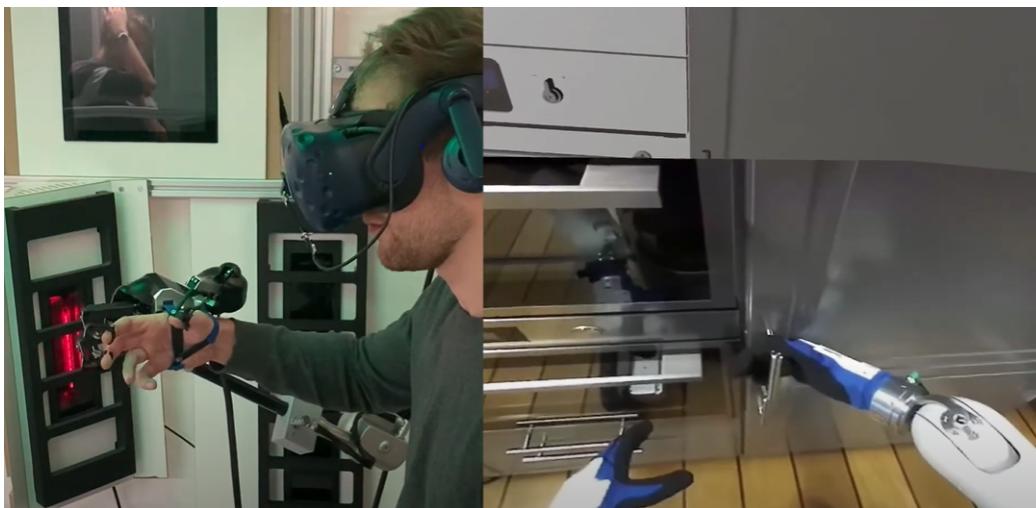
Figure 1.3: Perspective through Head Mounted Display (HMD): The operator's view as seen through the Head Mounted Display (HMD) while remotely controlling the EVE humanoid robot, immersing themselves in the telepresence experience.
